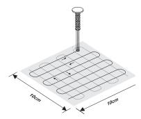
04. Hold the sampler vertically and insert into unibody, and fully depress to activate. **Note:** The sampler must be held vertically.
